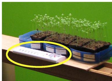
Placing the humidity meters side by side revealed that they tended to report slightly different humidities at the same time and place. I compared the humidity readings side by side on 3 days, and estimated that the average difference was only 1% (with a standard deviation of  $\pm 2\%$ ). I normalized the reported humidities accordingly.
